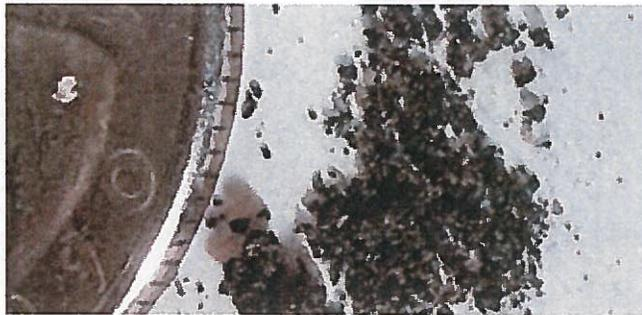
**Black Particles inside a Plant Cartridge Filter
